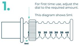
For further use adjust the dial in increments to the required amount.
